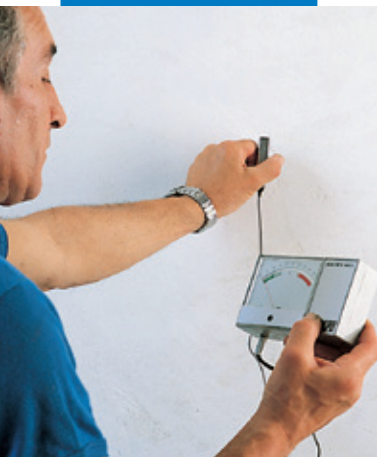
Checking gypsum plaster humidity
